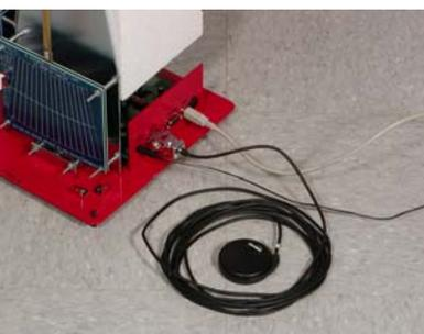
The GPS Receiver, inside the black disk at the end of the GPS assembly cable, requires radio frequency line of sight to the sky for proper operation. For optimal results, the GPS Receiver
