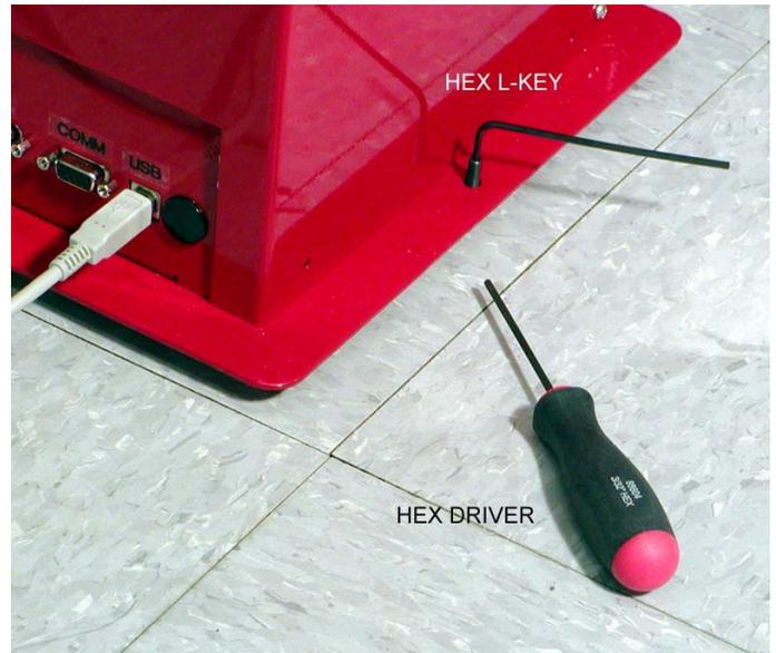
For more precise leveling than is possible with the Hex Driver in the tool kit, use the Hex L-Key with the long bar horizontal. The Hex L-key permits more precise movement of the Leveling Screws
