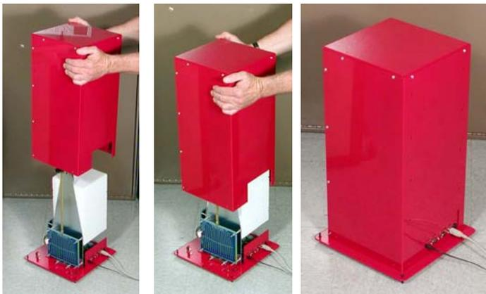
and the I/O Panel. If you do happen to nudge the VolksMeter slightly, it can be corrected with the Leveling Screws. It is normally not advisable to secure the Cover to the Base with screws at the permanent site. In fact, fastening the Cover screws will cause unnecessary deflection of the Base that will require more time to stabilize. Check the rough level. Re-adjust the Leveling Screws if necessary per section 2.6.
