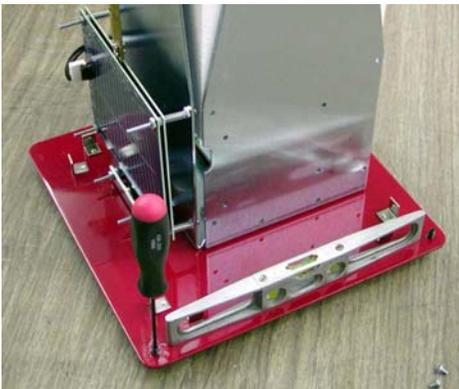
two in corners and one in the middle of the opposite edge. Place the level between the two corner screws first and adjust these screws as required to level that edge.
