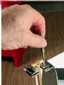
Once the moving plate is aligned with the fixed plates, check the Pivot Plate at the top of the Pendulum Rod.
