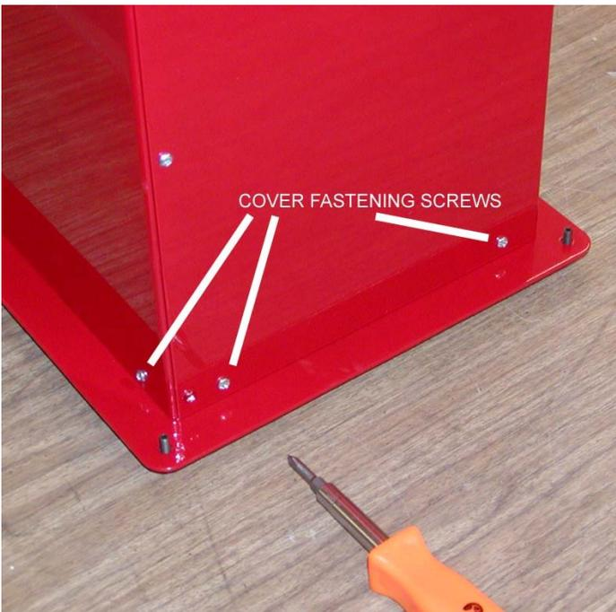
Use the Multi-tool to remove the screws that hold the VolksMeter Cover to the Base Plate. There are seven such screws located along the lower edge of the Cover. There are two screws on each side of the Cover except for the side with the I/O Panel, which has a single screw. Remove and save all seven screws.
