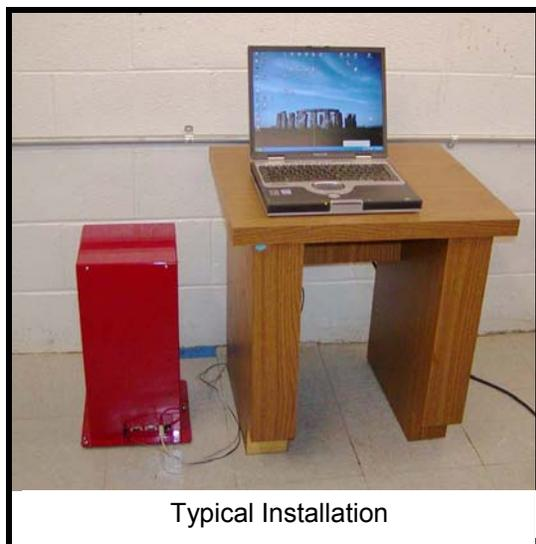
VolksMeter to access these leveling screws. Because of cable length limitations, the support computer must be located within 10 feet of the VolksMeter (a USB Booster may be used to increase this distance). The support computer may be controlled and monitored from a remote location via LAN (typically ethernet-based) and/or TCP/IP over the Internet using standard remote-access software.
